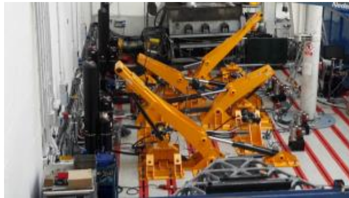
Fig. 1 Cyclist test of hydraulic cylinders
