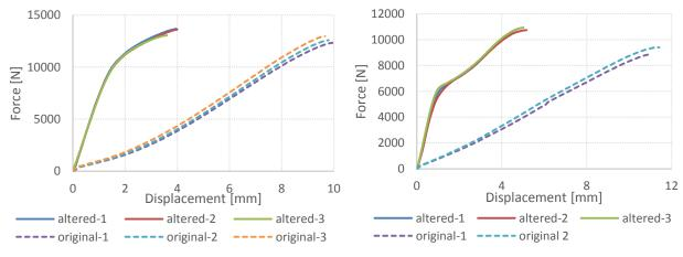
a) DOCOL 1200M, M5 size, Thickness 2mm b) S355J0, M6 size, Thickness 2mm
