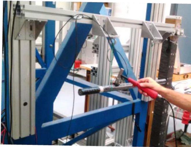
Fig. 4 Barrel sample fixation during EMA measurement.
