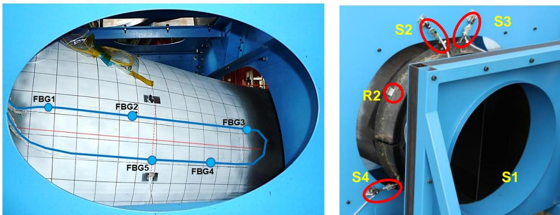
Fig.9 FBG (left) and strain gauge measurement (CTU) [10]
