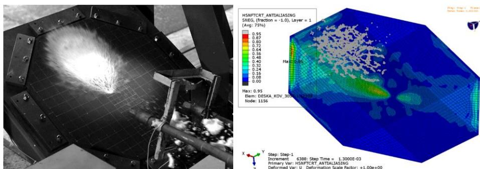
Fig.3 Hail stone impact test on flat test composite panel (left) and numerical simulation (right) [4]
