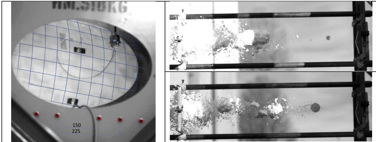
Fig.8 High speed camera pictures for deformation analysis in impacted area (left) and hail stone speed analysis (right upper - 25 mm ice ball; right bottom - 50 mm diameter ice ball)
