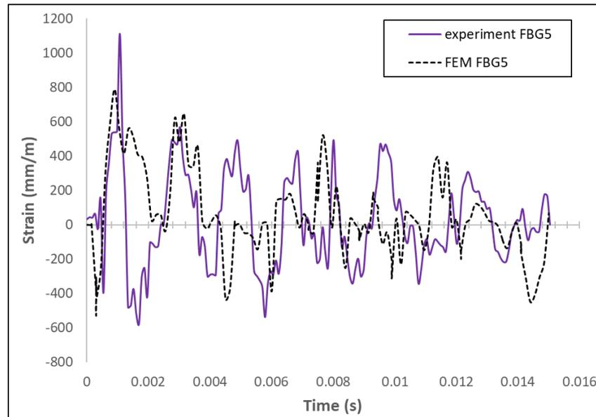
Fig.24 comparison between strain measurement on FBG sensors and numerical simulation for sensors FBG5 (see figure 9)
