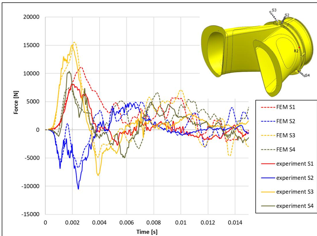
Fig.19 Comparison between experiment measurement of attachment rods load during impact and numerical simulation results. The results were compare for maximal peak of load.
