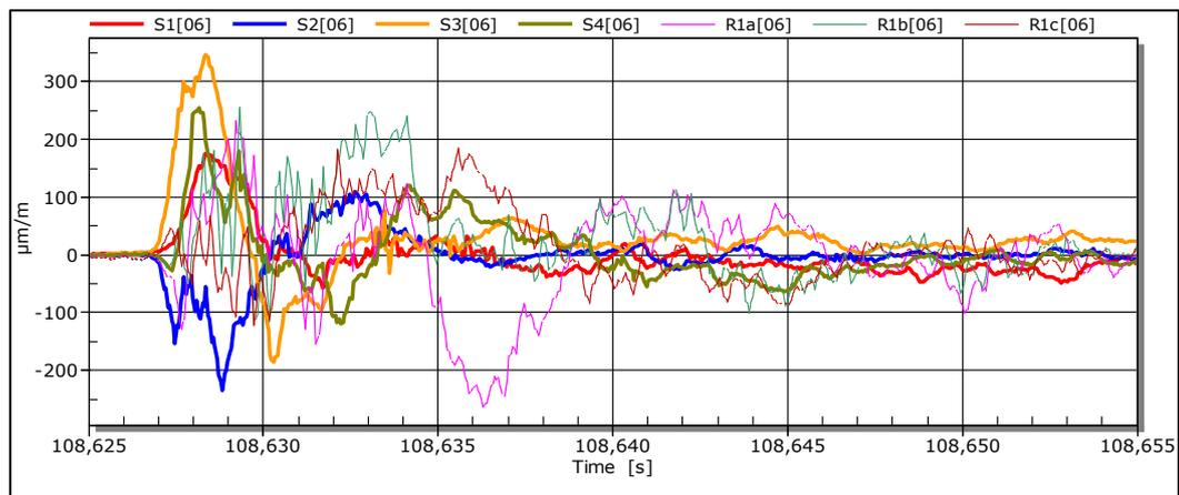
Fig.15 Strain gauge measurement during impact on attachment rods and attachment rig (CTU) (see figure 9) [10]
