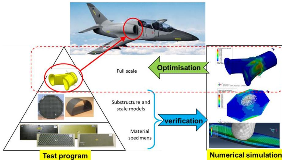
Fig. 1 Building block approach for testing and numerical simulation
