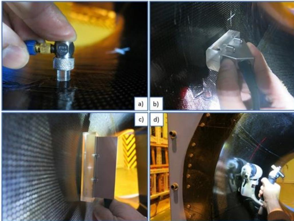
Fig.16 NDT measurement: a) Sonatest PRDT2550 probe; b) PA 5L64 probe; c) PA probe 2.25L128 and d) RolerForm 5 MHz.
