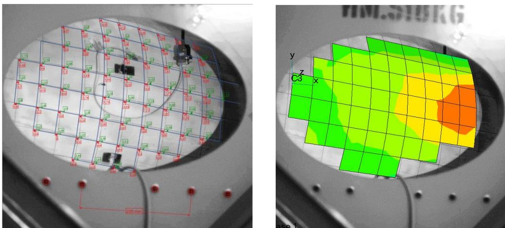
Fig.17 Analysis of displacement on the base of grid movement from high-speed camera pictures
