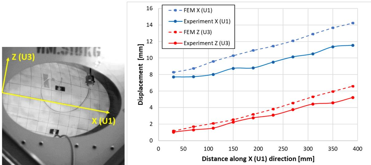
Fig.18 Comparison between qualitative measurement of displacement from high speed camera picture and numerical simulation for time impact 3 ms.
