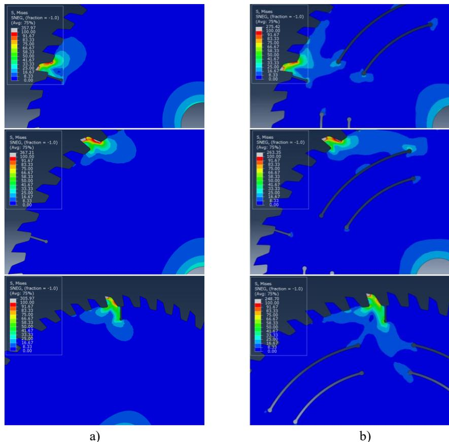
Fig. 3 Comparison of stress fields for: a) Conventional disc; b) an optimized disc
