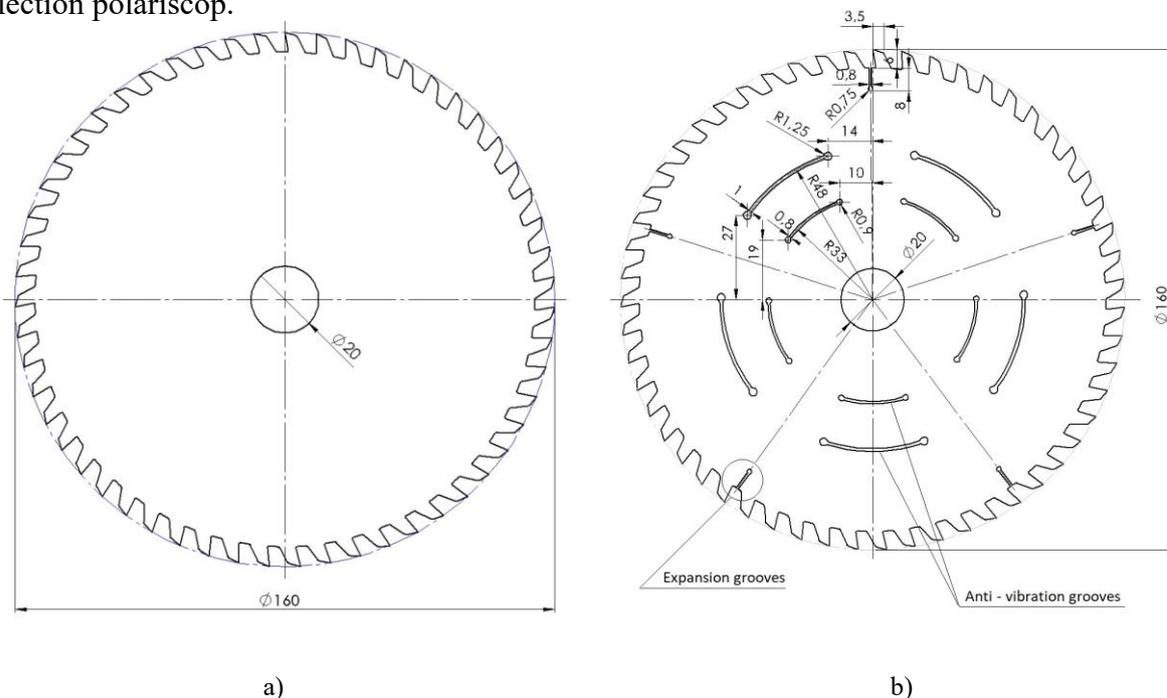
Fig. 2 The shape and dimensions of the saw blades: a) conventional; b) with anti-vibration grooves
