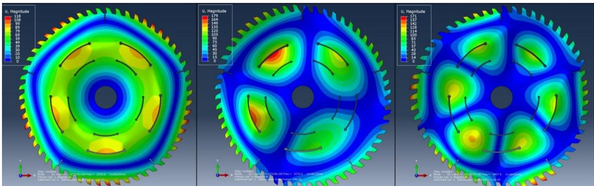
Fig. 5 Mode shapes of disc with anti – vibration grooves
