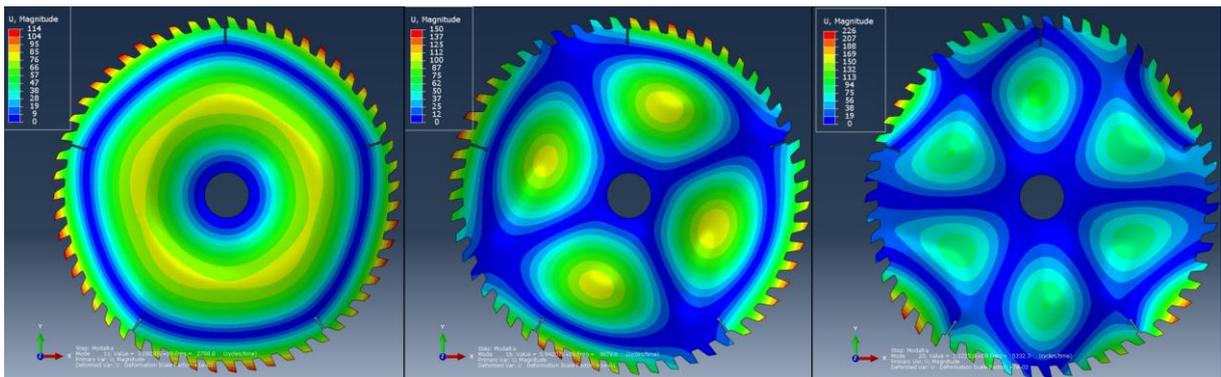
Fig. 4 Mode shapes of conventional disc
