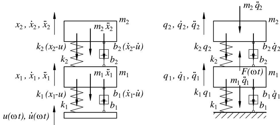
Fig.3 Description of system with two DOF
