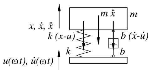
Fig.7 Description of system with one DOF
