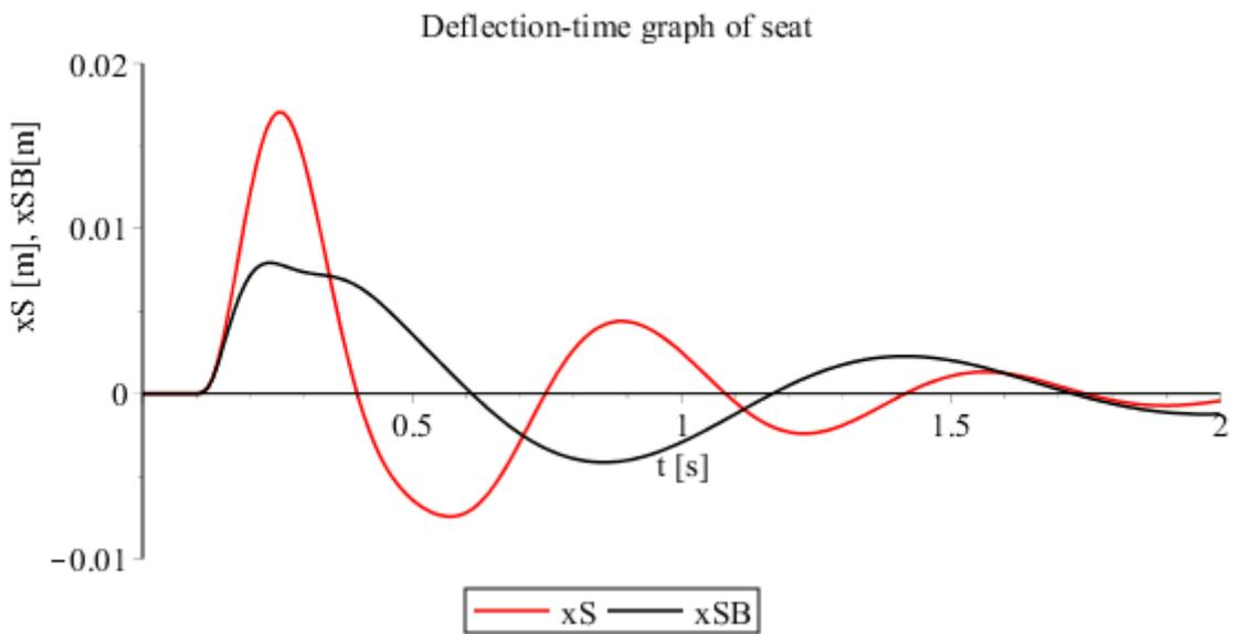
Fig.5 Step response of systems – deflection-time graph
