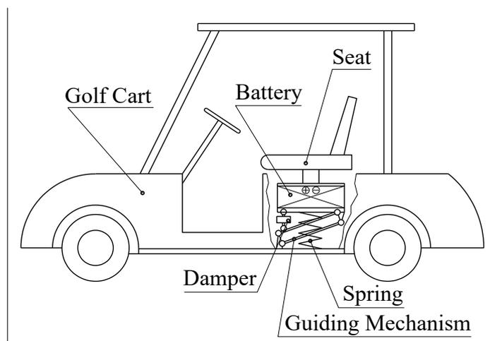
Fig.2 Principle of vibration isolation of seat
