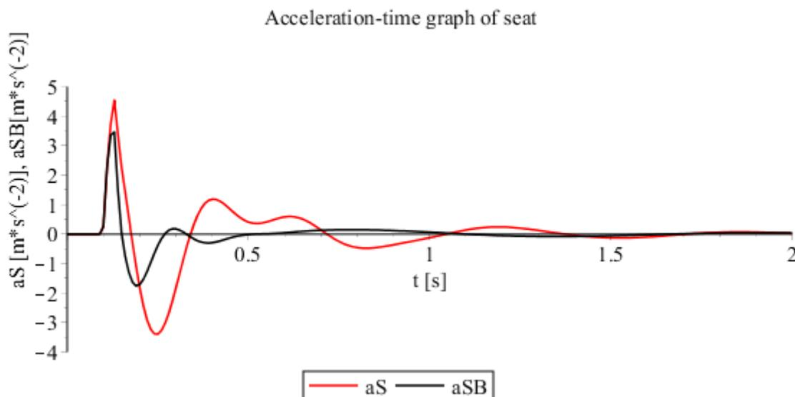
Fig.6 Step response of systems – acceleration-time graph
