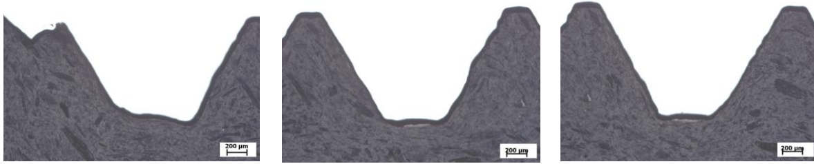
Fig. 9 Metallographic Cut of Threaded Surfaces of the M16 Nut (A4-80, with application of dry lubricant coating - “Gleitmo”). From the left side - 1. loaded thread, 2. loaded thread and 3. loaded thread. This photographs was processed by the corresponding author (2017)
