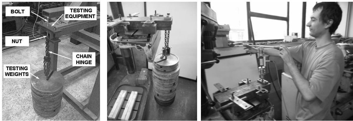
Fig. 5 Simple Testing Equipment for Evaluation of Threaded Contact Friction, (on the left side), HBM Torque Sensor T20WN, 20 Nm, (on the right side). These photographs were taken by the corresponding author (2015, 2016)
