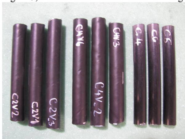
Fig. 5 Specimens group for torsion test
