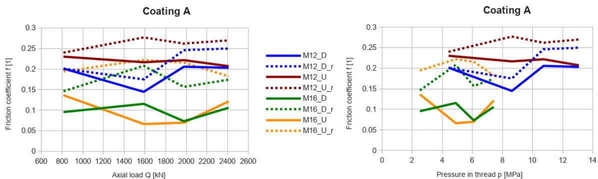
Fig 3 Friction dependence on axial load and pressure in the thread for coating A
