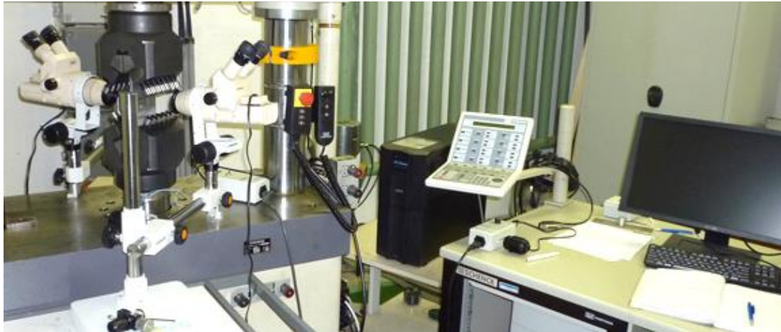
Fig.2 M(T) fatigue crack growth test configuration
