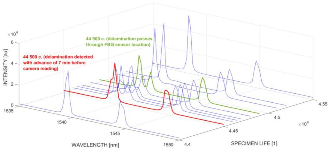
Fig. 50 Specimen MMB04 Bragg spectra reading, loaded state
