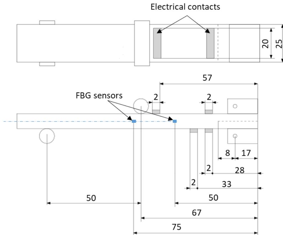
Fig. 47 Configuration of the electrical contacts and FBG sensors location
