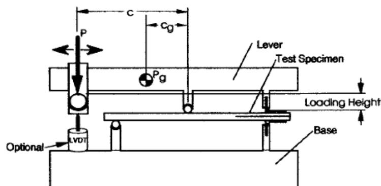
Fig. 48 MMB test configuration [7]
