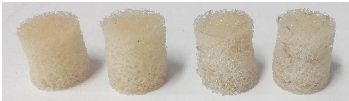
Fig. 2 Samples for DMA compression testing
