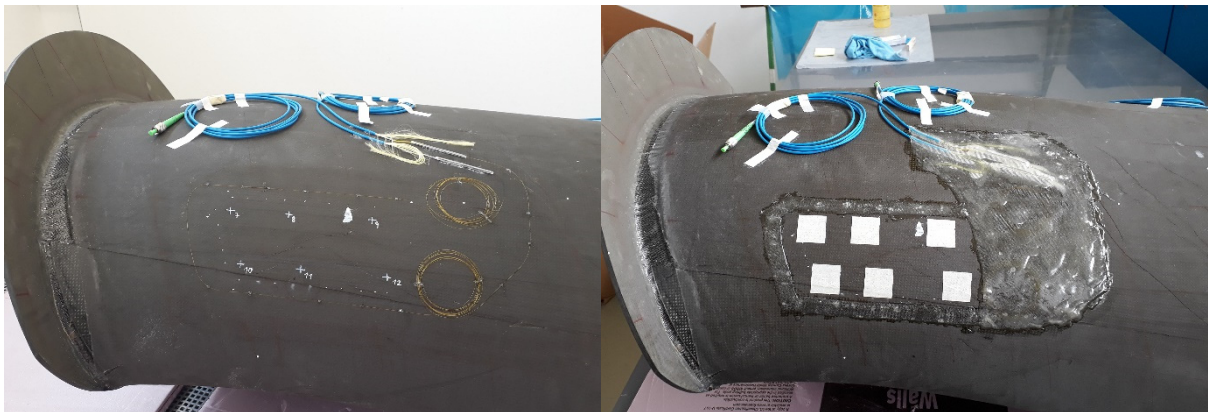
Fig. 2: Optical fiber with 6 FBG sensors attached to the air intake surface (left); optical fiber after lamination, before curing and painting (right)
