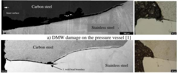
b) DMW damage on the piping system [2, 3] Fig. 1: Damage of DMW along diffusion line
