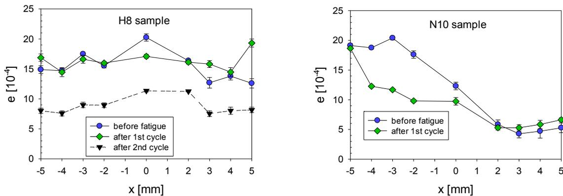
Fig. 4: Influence of high-cycle loading on the values of microdeformations on the UP side of samples, where  $x$  denote distance from the weld axis
