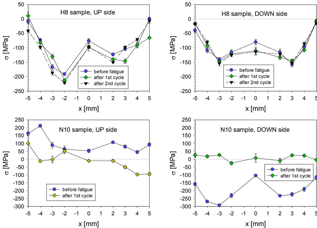
Fig. 3: Residual stresses in respect to the position from weld axis
