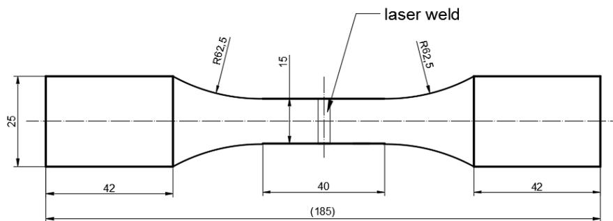
Fig. 1: Shape and dimensions of the fatigue test specimen
