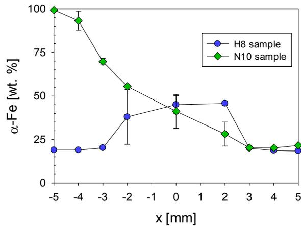
Fig. 5: Ferrite ( $\alpha$ -Fe) content in respect to the position from weld axis in the surface layers on the UP side of samples
