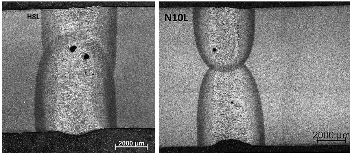
Fig. 2: Macrostructure of weld cross-section after etching
