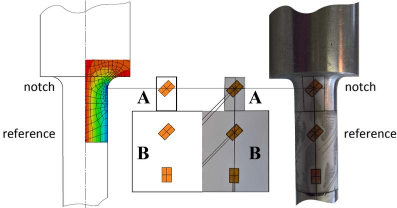
Fig. 3: Application foil design (left side) and use (right side – photo)
