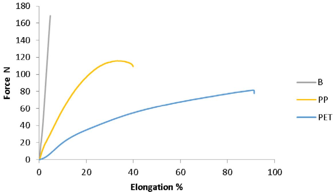
Fig. 1: Force & elongation curve for yarns
