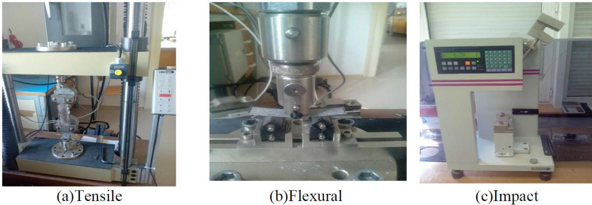
Fig. 2: Experimental set up for mechanical characterization of composites
