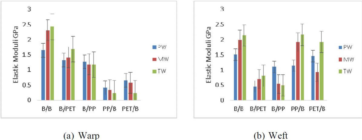
Fig. 3: Elastic moduli of composites
