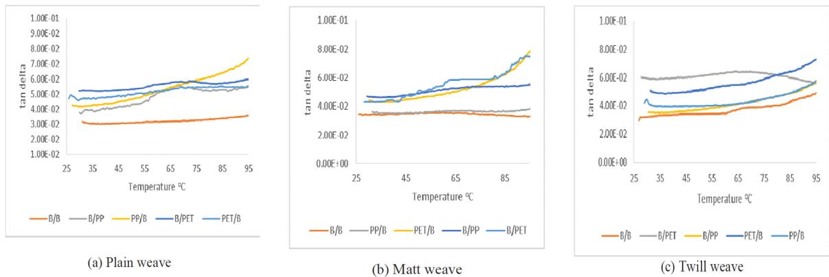
Fig. 7: Loss factor of all woven composites
