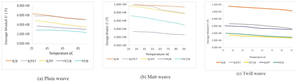
Fig. 6: Storage moduli for composites of all weaves
