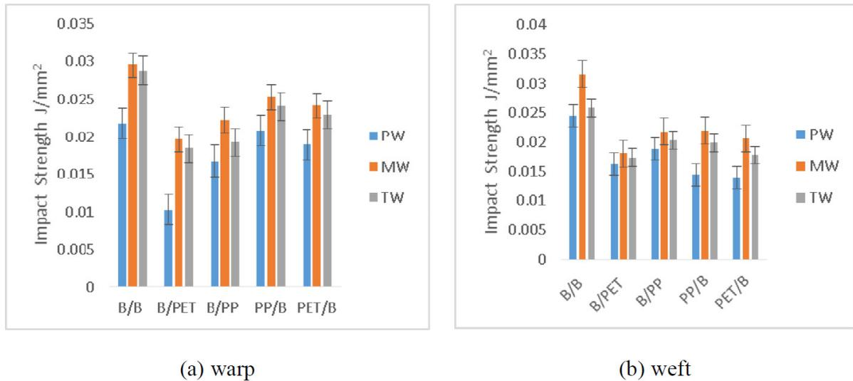
Fig. 5: Impact energy of composites
