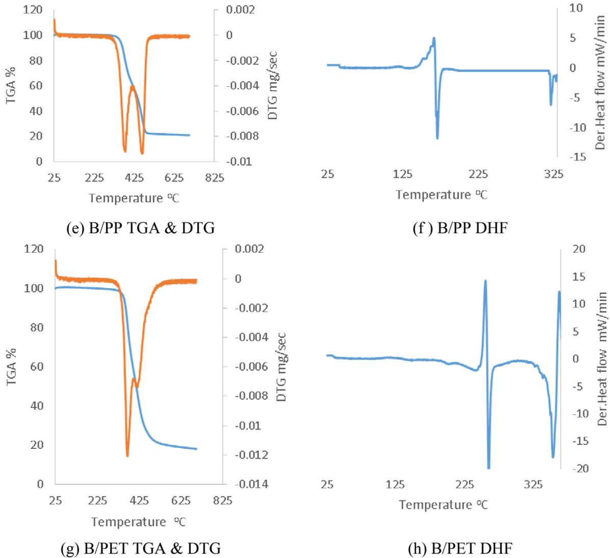
Fig. 9: TGA, DTG and DHF of specimens
