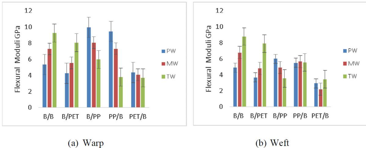
Fig. 4: Flexural moduli of composites
