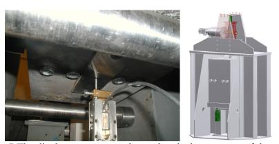
Fig. 7 The displacement sensor located at the bottom part of the stand
