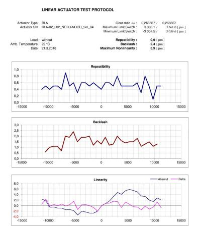
Fig. 6 Linear actuator test protocol without load
