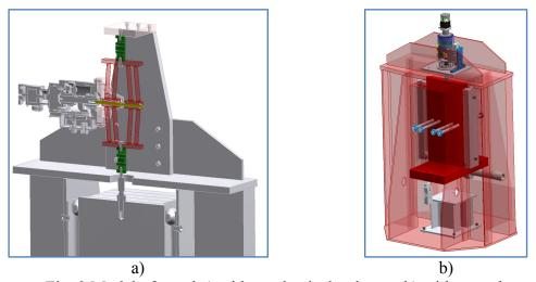
Fig. 3 Model of stand a) with mechanical reductor, b) without reductor
