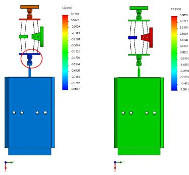
Fig. 2 Displacement fields of points in X and Y direction, respectively
