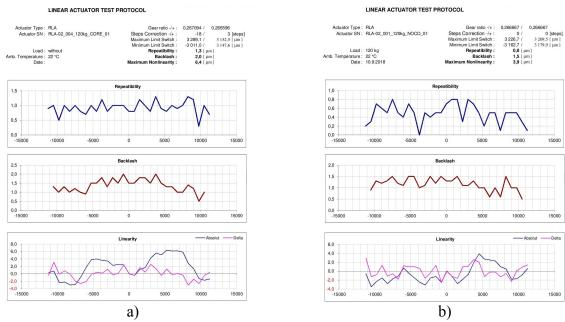
Fig. 8 Test protocol of actuator RLA a) without load, b) with load
