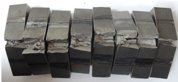
Fig. 5: Example of STRENX 700MC broken specimens after three-point bending fatigue tests
