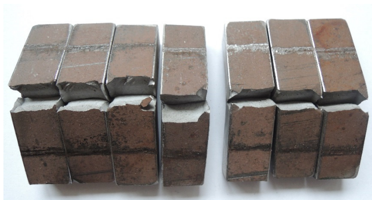
Fig. 5: Example of STRENX 700MC broken specimens after three-point bending fatigue tests
