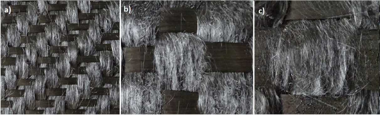
Fig. 4: Damage of elementary fibres after test; a) standard tow, b) flat tow, c) spread tow
