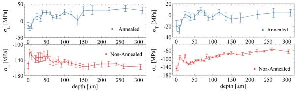
Fig. 2: Longitudinal L (parallel to the weld axis) and transversal T (perpendicular to the weld axis) RSs with respect to depth under the surface
