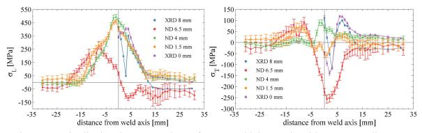
Fig. 5: Longitudinal and transversal RSs for 8 mm thick sample with respect to distance determined across the weld for different depths
