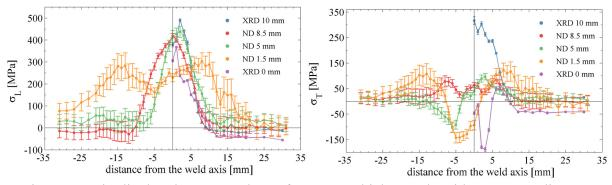
Fig. 4: Longitudinal and transversal RSs for 10 mm thick sample with respect to distance determined across the weld for different depths
