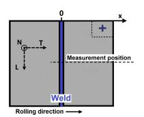
Fig. 1: Scheme of the sample. The cross in the right upper corner denotes the place where the depth profile was measured
