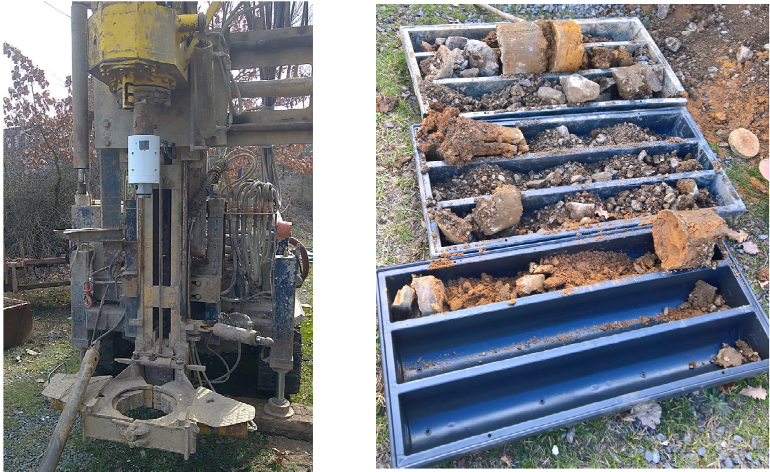
Fig. 6: Drilling in Zbraslav – drilling machine RDBS (left), 7.5 m drilled core (right)
