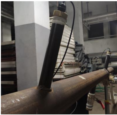
Fig. 11: Experimental setup for sensing of negative pressure wave
