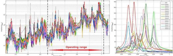
Fig. 7: Spectra measured with accelerometers at the root of leading edges
