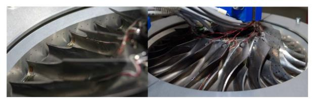
Fig. 5: Placement of the strain gauges on the trailing edge of the impeller blades and accelerometers on root of leading edges
