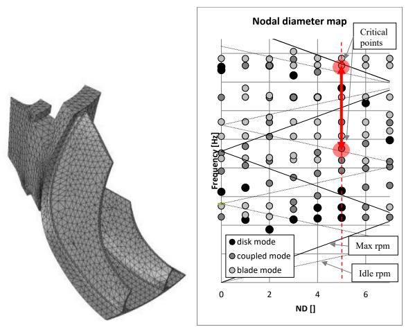
Fig. 2: a) FE model segment of centrifugal compressor and b) SAFE diagram
