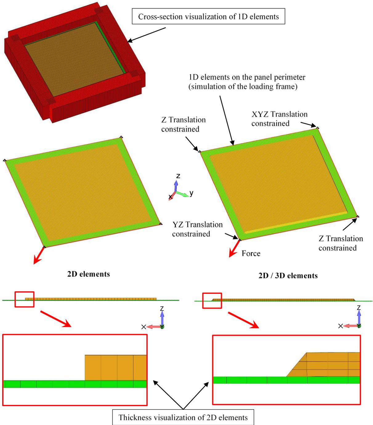
Fig. 4: FE models of sandwich panel
