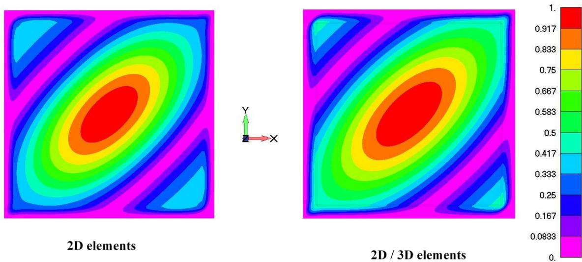
Fig. 8: The first eigenshape of the sandwich panel
