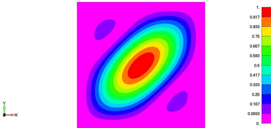
Fig. 9: The first eigenshape of the monolithic laminate panel
