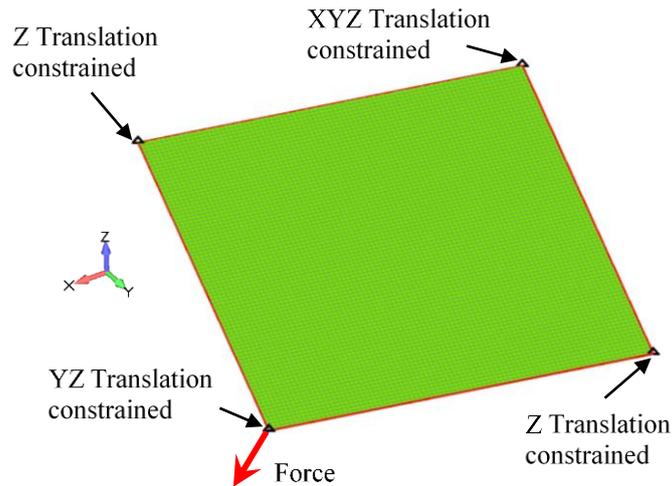
Fig. 5: FE model of monolithic laminate panel
