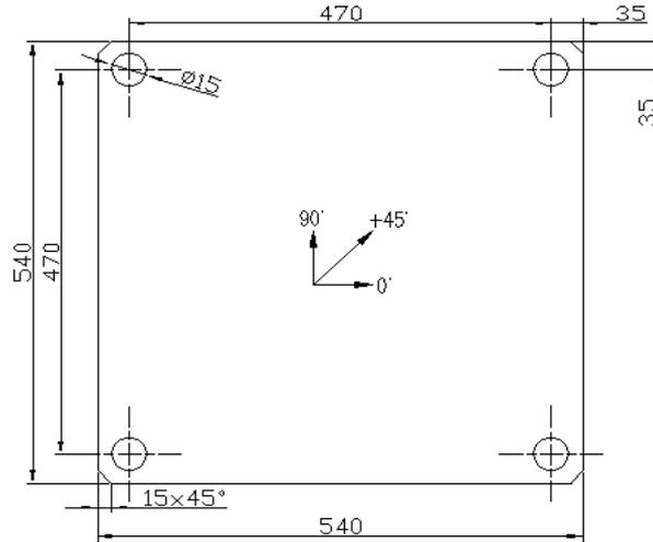
Fig. 3: Tested monolithic laminate panel [4]
