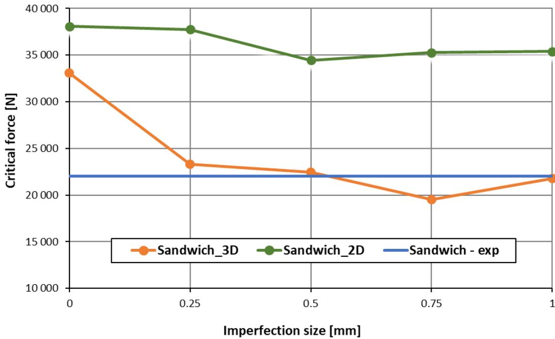
Fig. 11: Dependency of critical force on imperfections size – sandwich panel
