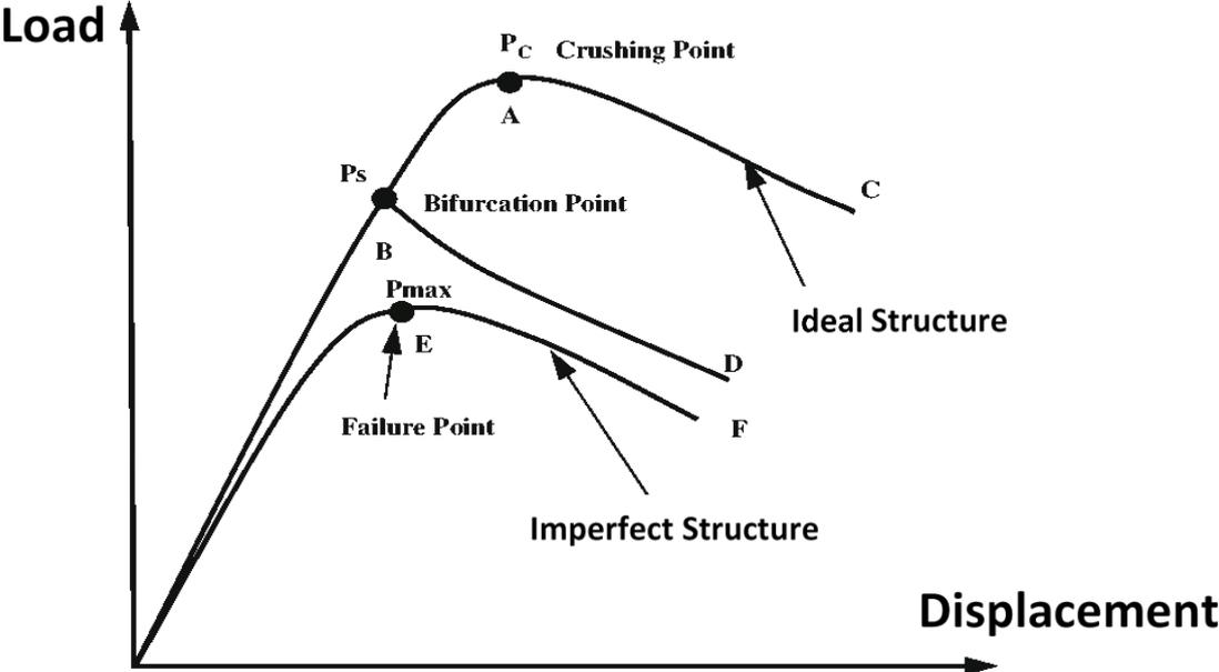
Fig. 1: Equilibrium paths for linear and nonlinear buckling [3]
