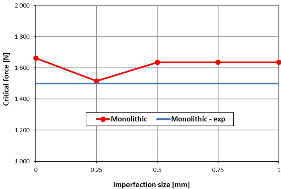
Fig. 12: Dependency of critical force on imperfections size – monolithic panel
