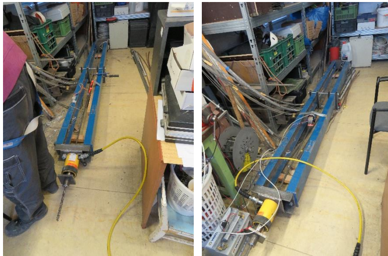
Fig. 4: View of arrangement of the experiments with the hollow hydraulic jack, the steel test frame, the fastened prestressed strand and the first variant of the removable elastomagnetic sensors attached to the strand (on left) and the second one (on right)
