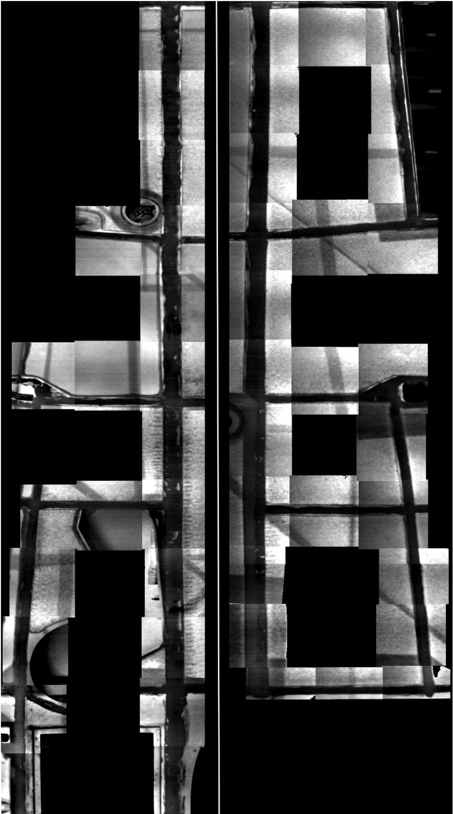
Fig. 8: Results of PT NDE method – overview image of the tested wing area (lower wing side on the left, upper wing side on the right)
