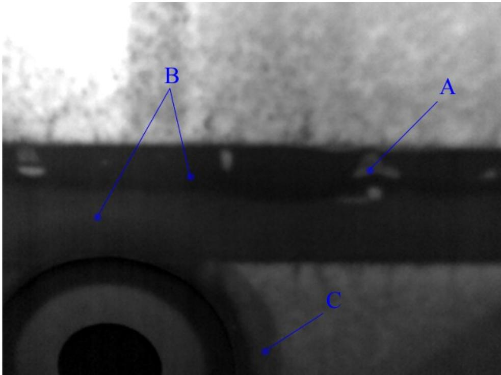
Fig. 6: Results of PT NDE method – adhesive joint of the front wing spar and the upper wing skin in the fuel tank area
