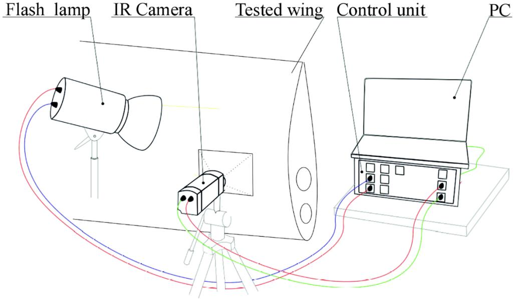
Fig. 4: Experimental configuration
