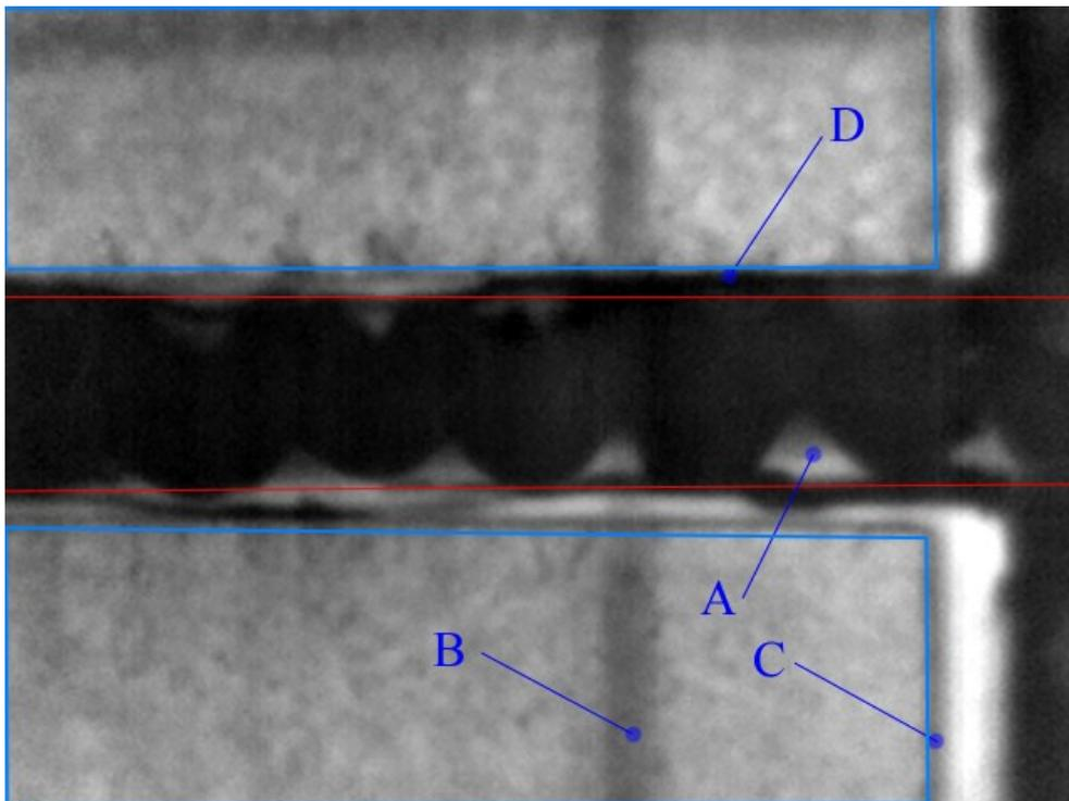
Fig. 5: Results of PT NDE method – adhesive joint of the front wing spar and the wing tip rib on the lower wing skin
