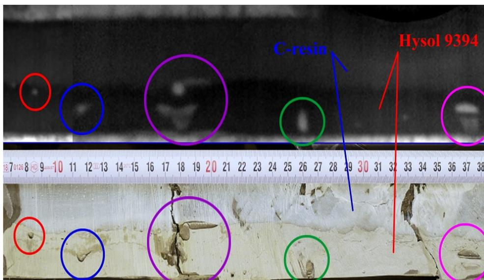
Fig. 7: Comparison of NDT findings (top) with the actual condition of the adhesive joint (bottom)
