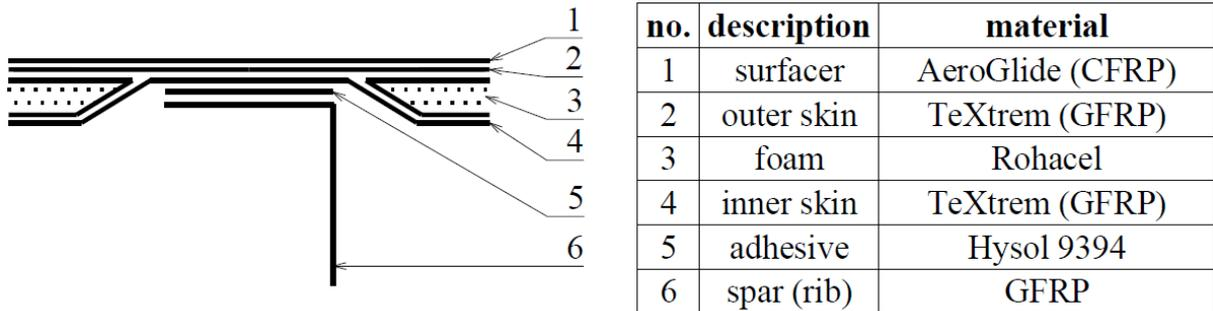
Fig. 1: Bonded joint configuration
