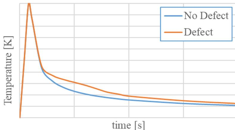
Fig. 2: Surface cooling curves
