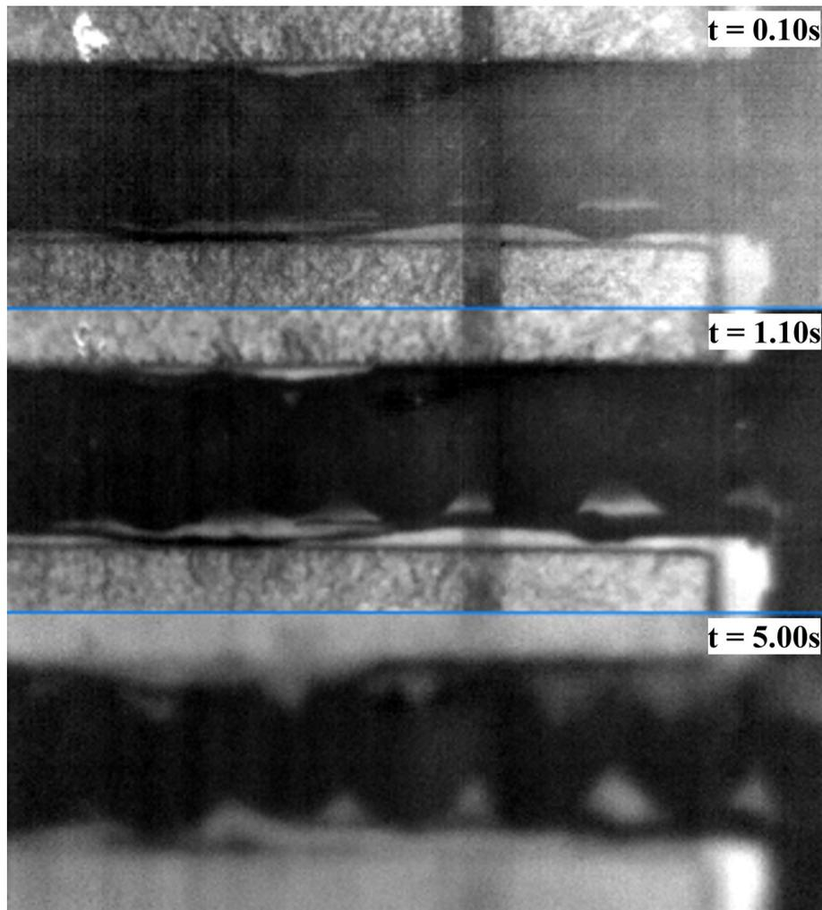
Fig. 3: Sequence of thermograms of the bonded joint
