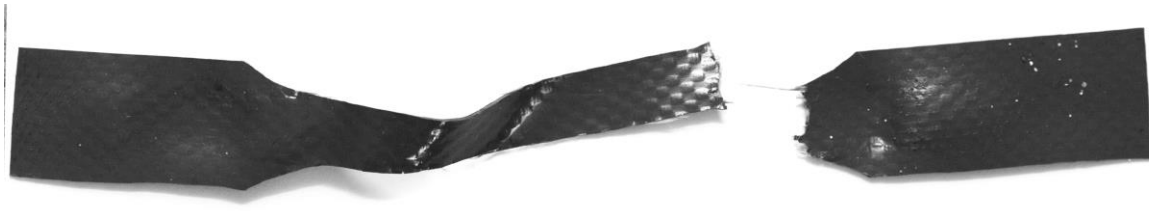
Fig. 8: Failure example in the warp direction
