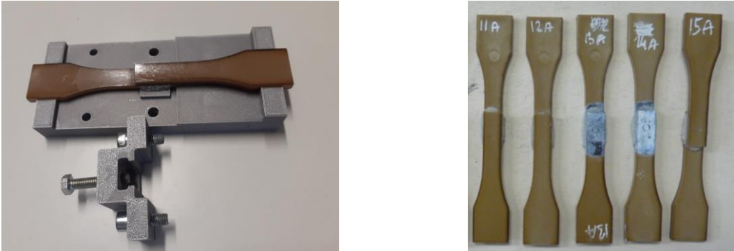
Fig. 2: Test specimen in the jig after gluing (left figure) and final test specimens before testing (right figure)
