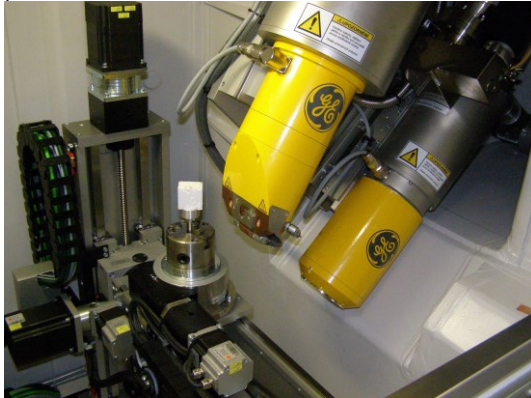
Fig. 3: Phoenix v|tome|x s 240 inspection equipment - 240 kV 320 W micro-focal open X-ray tube and 180kV high-performance nano-focal X-ray tube
