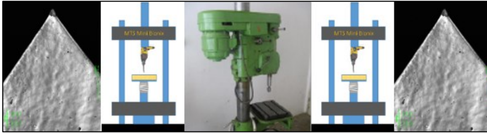
Fig. 1: One cycle of the experiment: 1. Olympus LEXT OSL 3000, confocal microscope, photo and profile; 2. MTS 858.02 Mini Bionix, measured F , M ; 3. Defined drilling wear, 40 cycles or 8 cycles; 4. MTS 858.02 Mini Bionix, measured F , M ; 5. Olympus LEXT OSL 3000 confocal microscope, photo and profile
