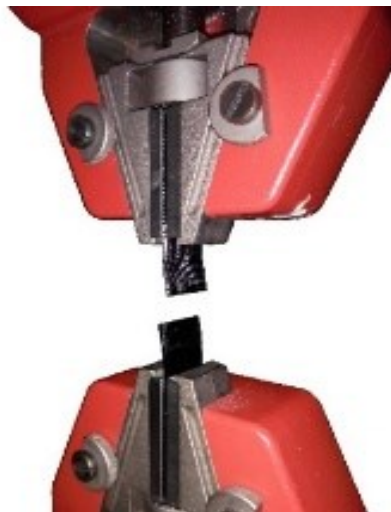
Fig. 2: Sample clamped in to testing device after tensile test,
