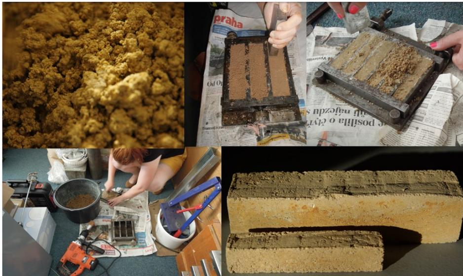
Fig. 1: Producing the mixture and final specimens
