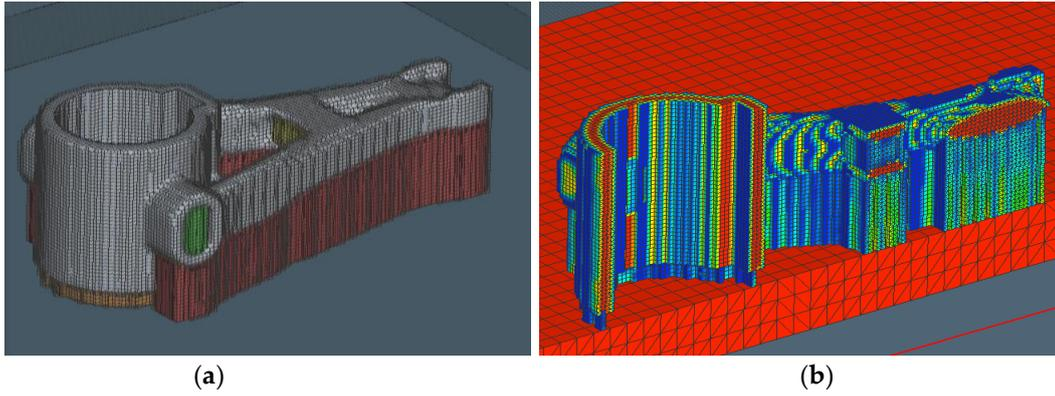
Fig. 5: Voxel and Surface mesh (a); Voxel mesh analysis (b)
