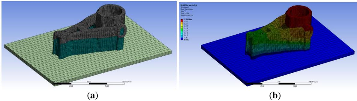
Fig. 3: AM meshing for thermal analysis (a); thermal analysis results (b)
