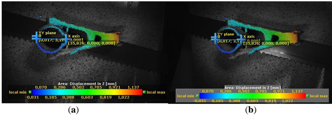
Fig. 7: Maximum displacement on the left camera (a) and on the right camera (b)
