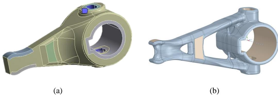
Fig. 2 Original geometry of main shifting thumb (a); Topologically smoothed shifting thumb (b)
