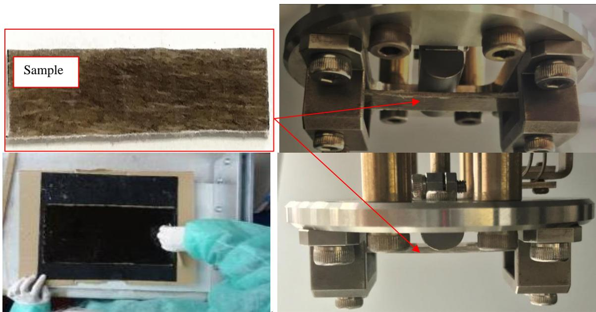
Fig. 2: Preparing of sample 50mm×10mm×1.35mm (left), device for experiment (right)
