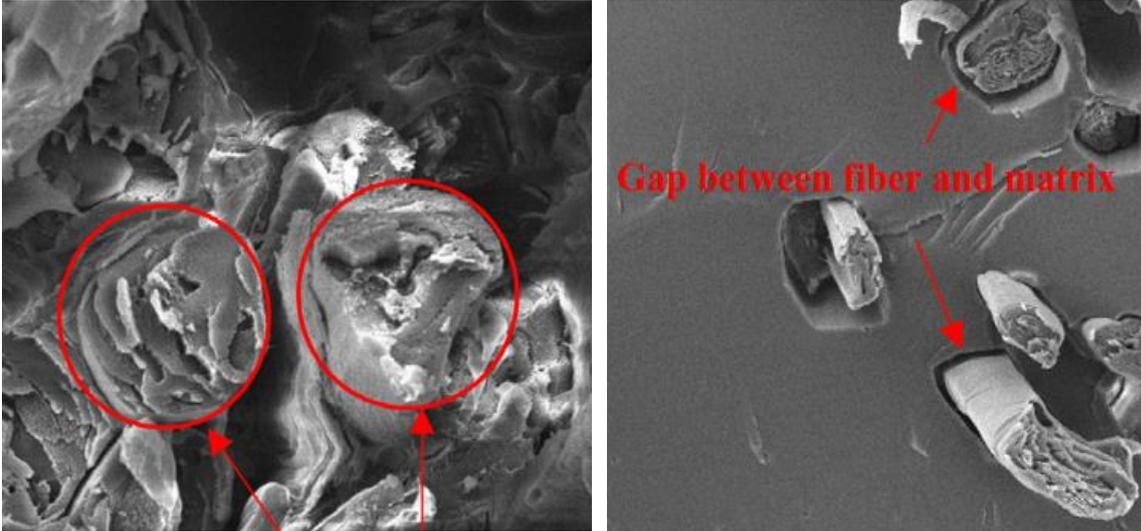
Fig. 4: Detail of morphology structure of FFRP sample: before under accelerated aging (left), after 167.8 hour under accelerated aging (right)
