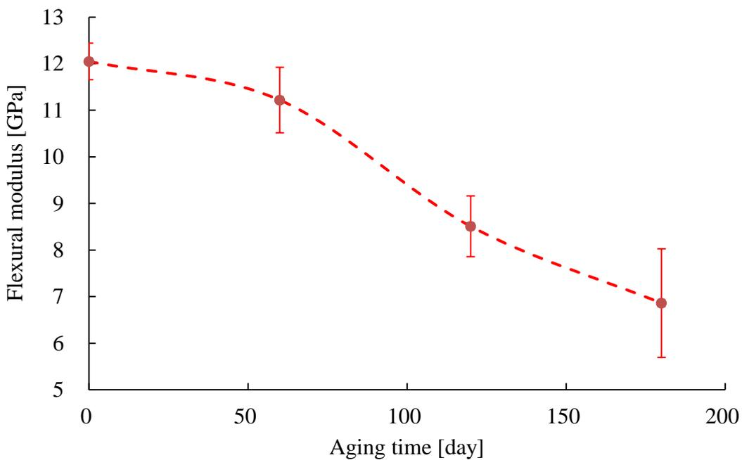
Fig. 1 Results of bending properties of FFRP under accelerated aging: (above) flexural strength, (below) flexural modulus
