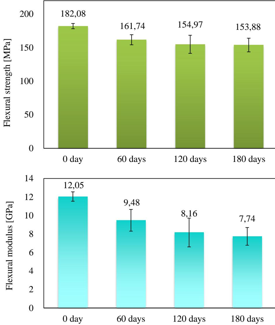
Fig. 1: Bending properties of FFRP after natural aging: (above) Flexural strength, (below) Flexural modulus
