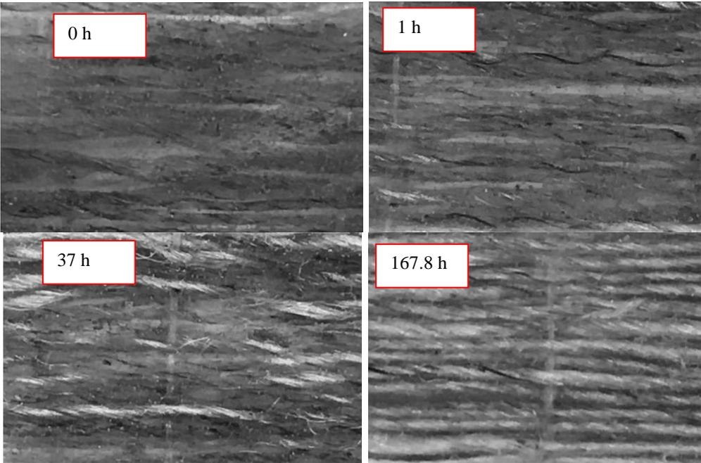
Fig. 3: Damage of sample of FFRP under accelerated aging
