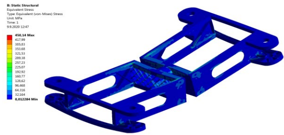
Fig.9: Reduced stress in the composite frame
