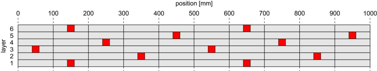
Fig. 2 Scheme of locations of layer separations indicated by red marks. Layer 1 is at the inner diameter and layer 6 is at the outer diameter.
