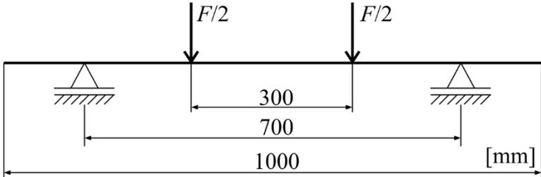
Fig. 3 Scheme of the four-point bending test.
