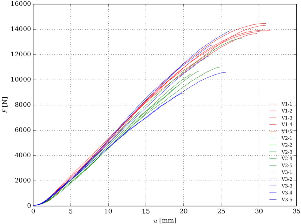
Fig. 4 Measured force–displacement dependencies for all tested tubes.
