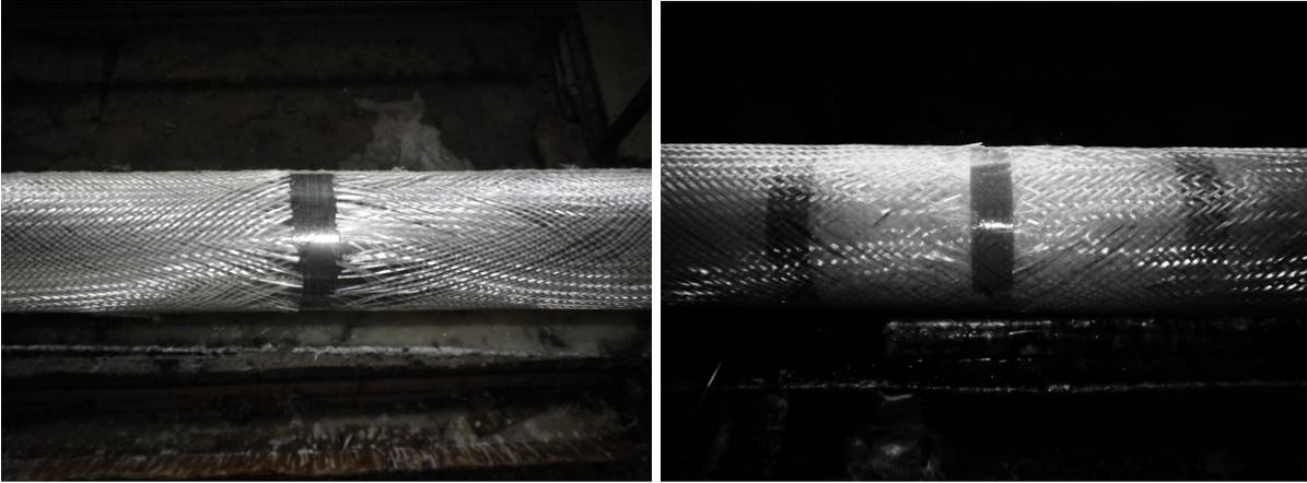
Fig. 1 Example of Kapton tape applied in the first layer (left) and in three different layers (right).
