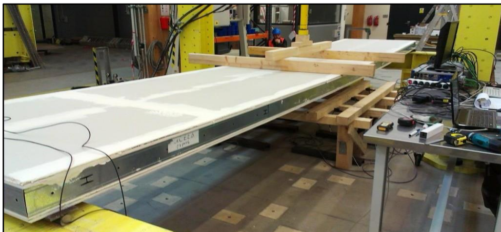
Fig. 2: Set up of experimental verification of the bending stiffness of the wall panel.
