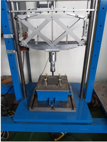
(a) Impact test setup
