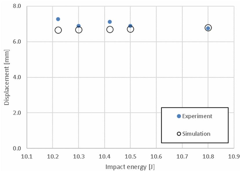
Fig. 3: Vertical displacement (laminates deflection) under impactor.
