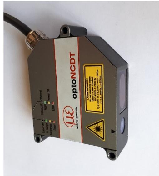
(b) Laser interferometer optoNCDT ILD 2300-20
