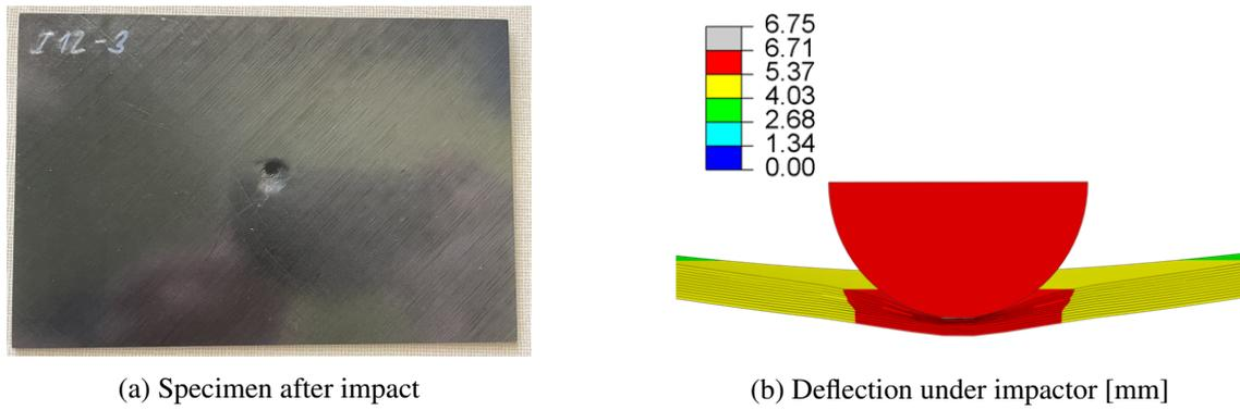
Fig. 2: Real and modelled damage.
