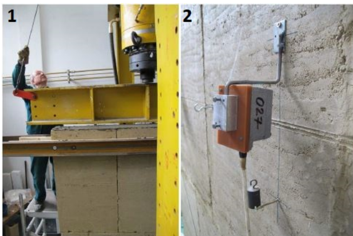
Fig. 6: 1) The setting of the steel beam and position of the load cell with the hydraulic jack and 2) the gauge for recording local strain [1].
