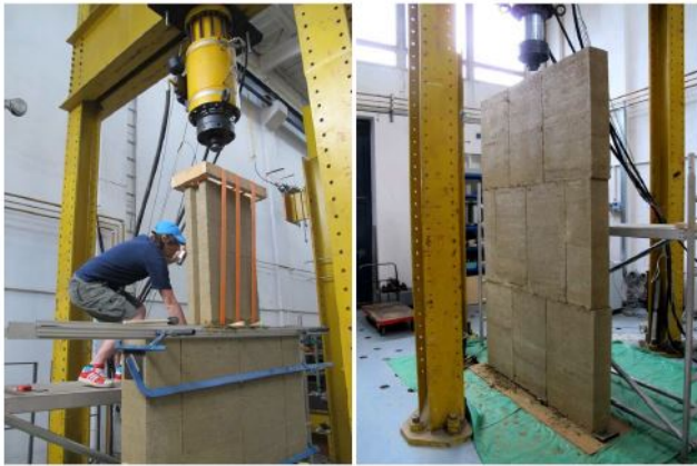
Fig. 1: Precast earth wall [1].
