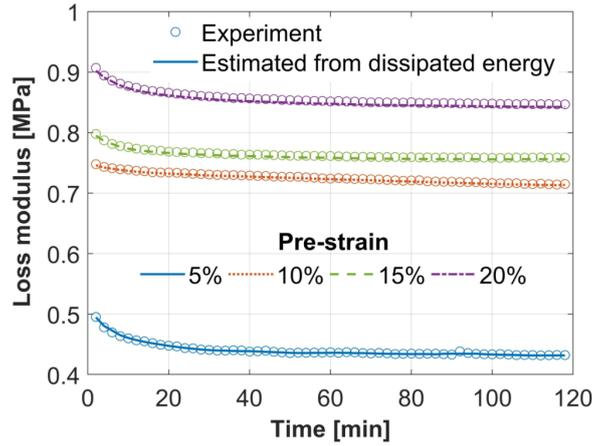
Fig. 3: Loss moduli of the MEC determined from recorded signals according to Eq. 7 and estimated from the dissipated energy by Eq. 8 as functions of time and pre-strain.
