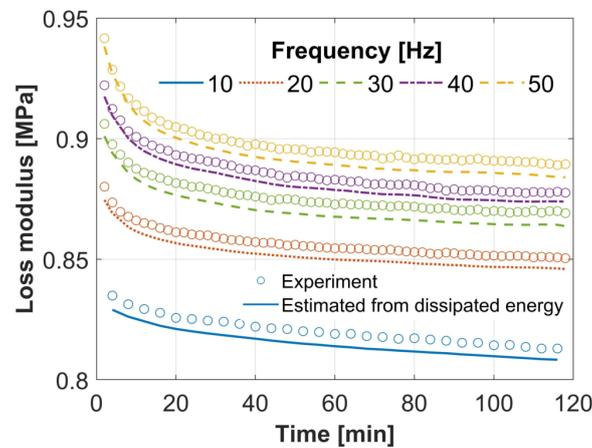
Fig. 5: Loss moduli of the MEC determined from recorded signals according to Eq. 7 and estimated from the dissipated energy by Eq. 8 as functions of time and strain amplitude.
