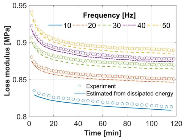
Fig. 7: Loss moduli of the MEC determined from recorded signals according to Eq. 7 and estimated from the dissipated energy by Eq. 8 as functions of time and frequency.
