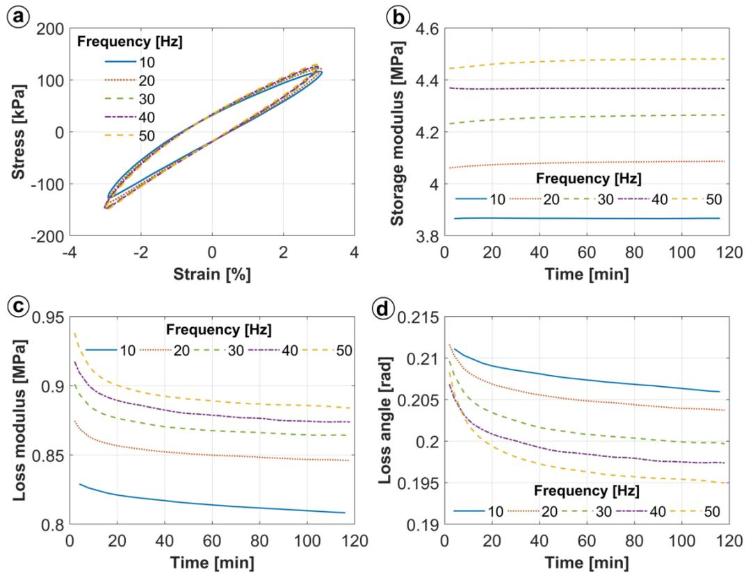
Fig. 6: (a) Typical stress-strain hysteresis loops; (b-d) storage and loss moduli, and loss angle of isotropic MEC under cyclic loading with the pre-strain of 20%, the strain amplitude of 0.03, and different frequencies.
