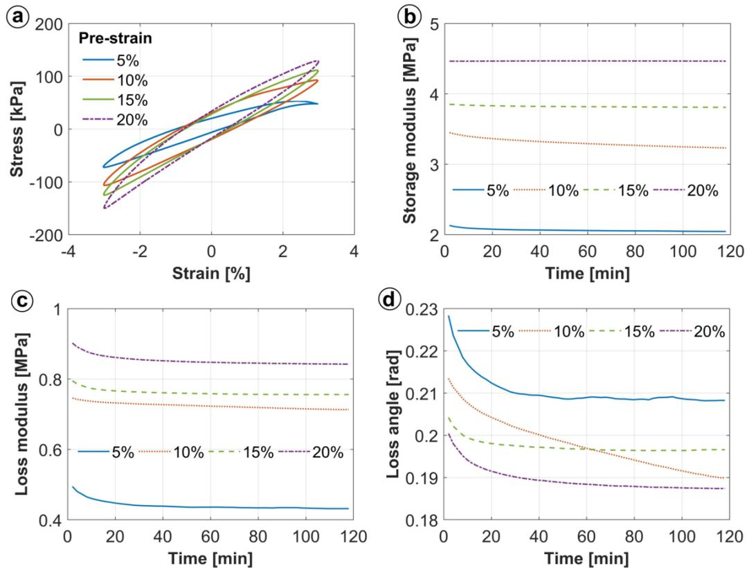
Fig. 2: Typical stress-strain hysteresis loops; (b-d) storage and loss moduli, and loss angle of isotropic MEC under cyclic loading with the frequency of 50 Hz, the strain amplitude of 3%, and various pre-strains.
