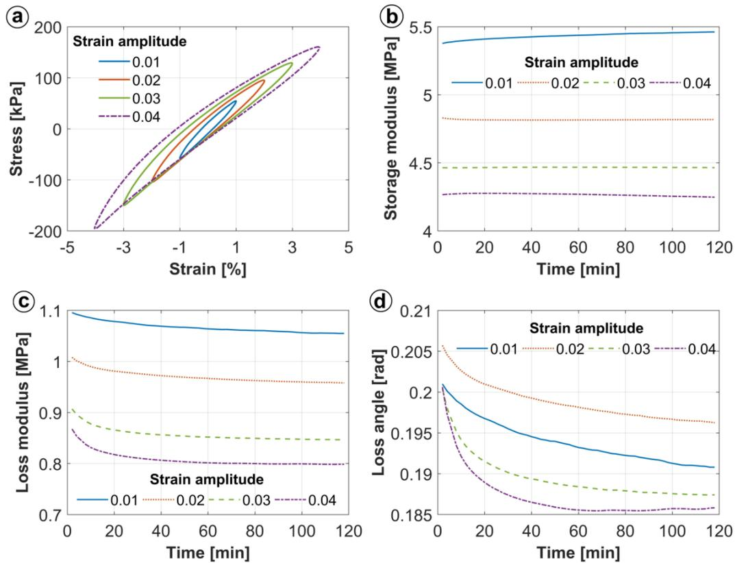
Fig. 4: (a) Typical stress-strain hysteresis loops; (b-d) storage and loss moduli, and loss angle of isotropic MEC under cyclic compression loading with the frequency of 50 Hz, 20% pre-strain, and different strain amplitudes.
