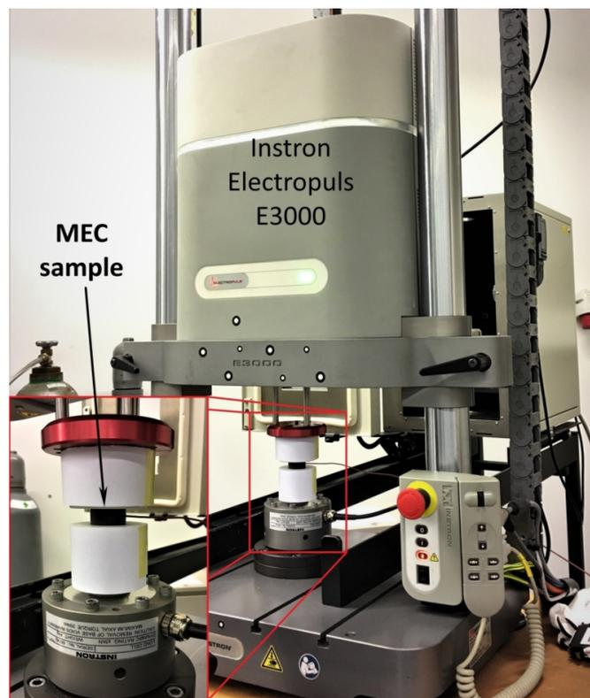
Fig. 1: The experimental setup of cyclic compression test for the MEC samples.
