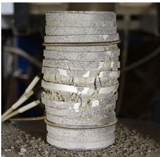
Fig. 1: The cylinder specimen after compression test. The specime was tightened with 12 rings thickness 2 mm.
