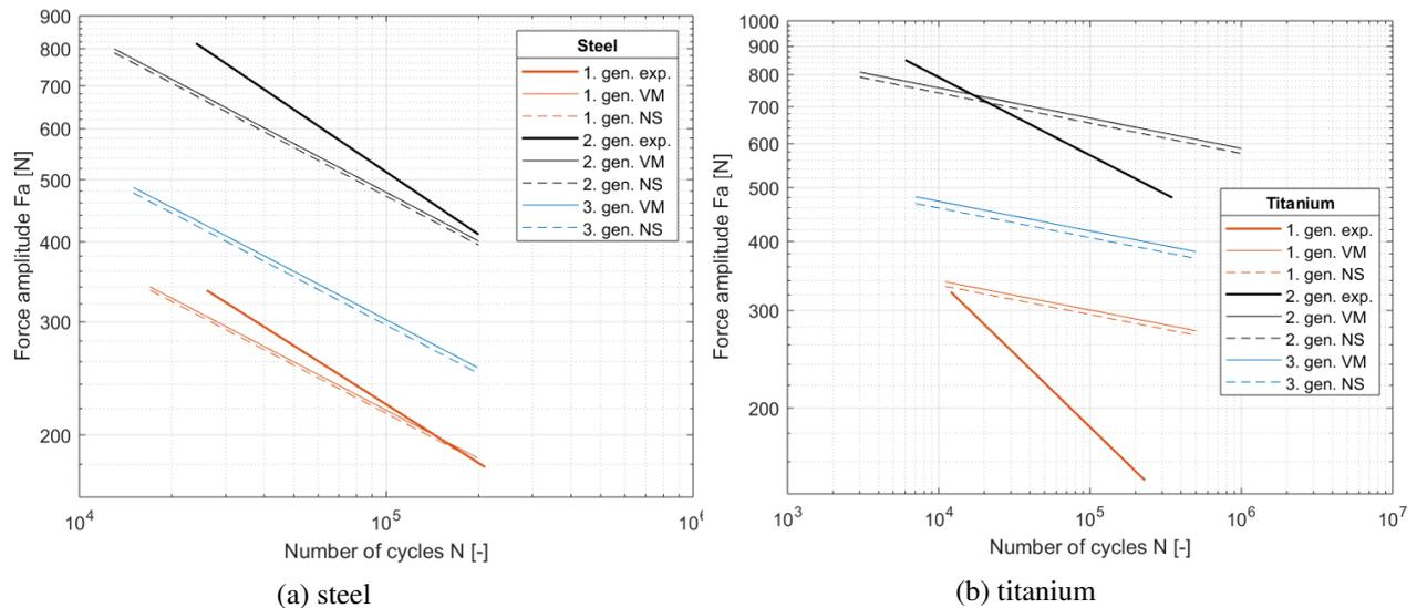
Fig. 4: Comparison of experiments and fe-safe results for all generations in stress amplitude.
