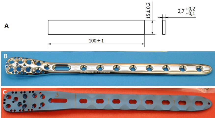
Fig. 1: (A) Dimensions of the flat sample for the four-point bending test, (B) stainless steel bone plate of the first generation, (C) titanium alloy bone plate of the second generation.
