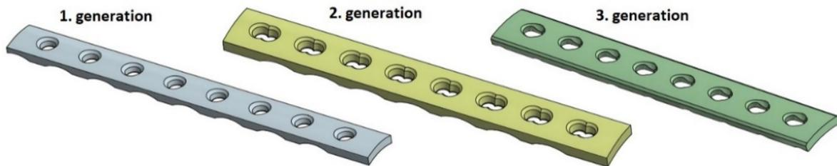
Fig. 2: Models of three generations of bone plates.
