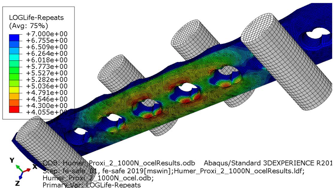
Fig. 3: Results of the fe-safe analysis for the second generation of steel bone plates displayed as a contour plot in Abaqus.
