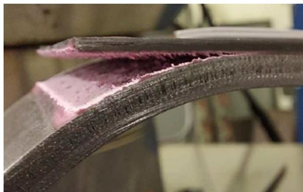
Fig. 13: Detail of debonding of the reinforce end after plastic deformation of the beam.
