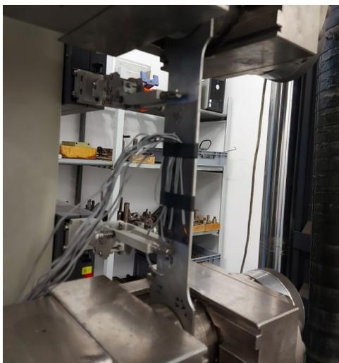
Fig. 5: DSR specimen under static tensile test.
