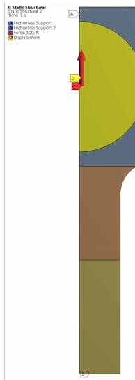
Fig. 9: Loading and boundary conditions of the  $\frac{1}{4}$  test specimen FEM model.
