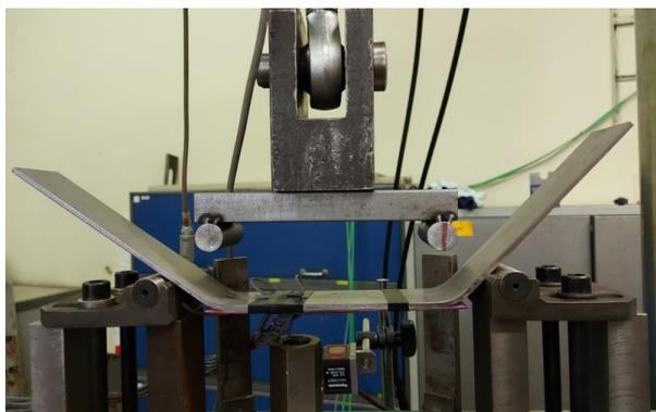
Fig. 12: Four-point bending test of steel plate with glued CFRP plate. Plastic joints on both reinforced ends and visible debonding of the CFRP plate.
