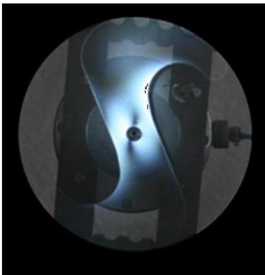
(a) Field of isochromatics at angular velocity  $\omega = 125.7 \text{ rad}\cdot\text{s}^{-1}$ .
