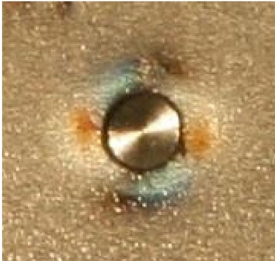
(a) Field of isochromatics around a blind cylindrical hole with a depth of 0.3 mm.
