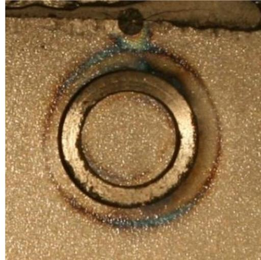
(b) Field of isochromatics around a groove with a depth of 2.0 mm for the Ring-Core method.
