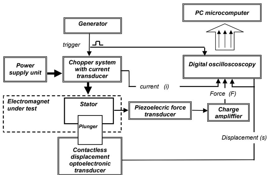
Fig. 5. Testing of the dynamic characteristics of the miniature linear electromagnet
