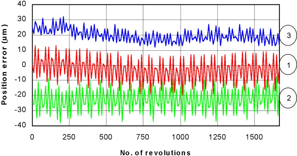
Fig. 2. Kinematic deviation of the screw position and hysteresis for drive unit *B*
