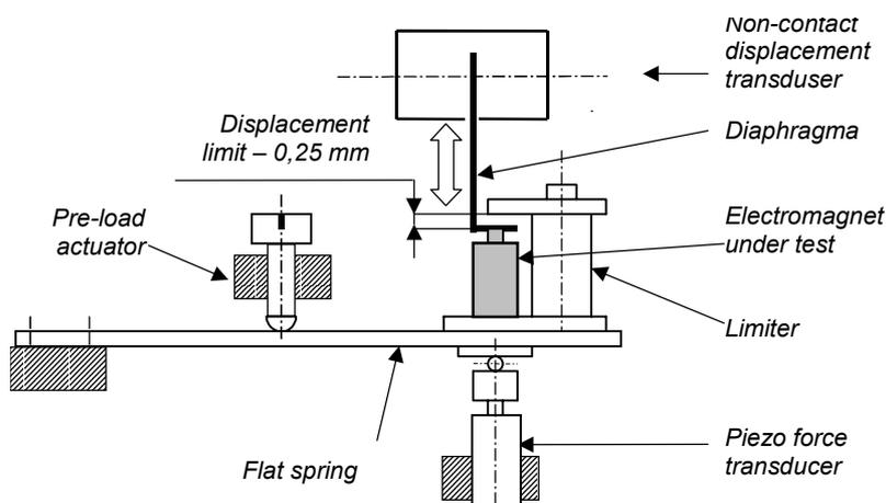
b) structure of the mechanical unit of the test station
