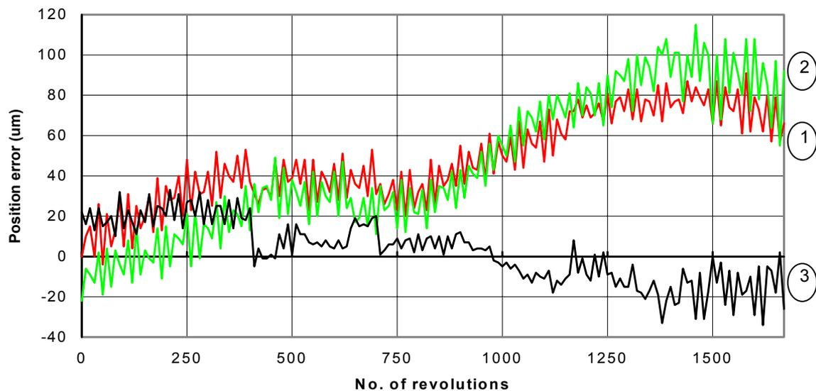
Fig. 1. Kinematic deviation of the screw position and hysteresis for drive unit *A*
