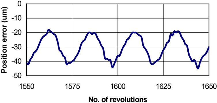
Fig. 3. Cyclical variations of the kinematic deviation of the screw position for drive unit *B*
