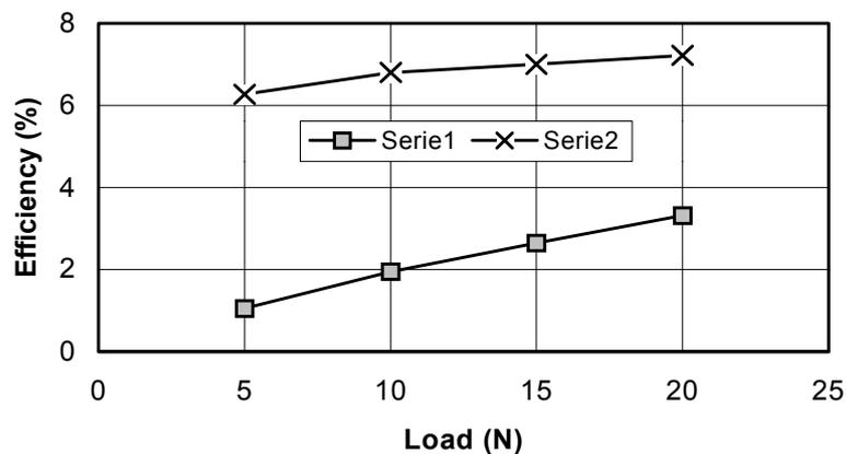
Fig. 4. Efficiency of the linear drive (Series 1) and toothed gear coupled with screw gear (Series 2)
