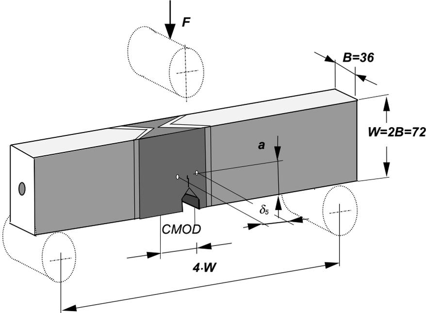
Figure 2. Three point bending specimen ( $B \times 2B$ ) and measuring points (CMOD,  $\delta_5$ )
