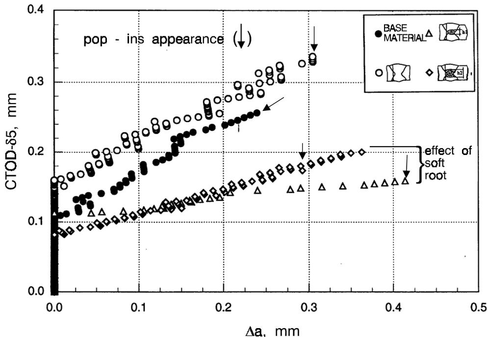
Figure 5. Resistance curves for specimens (B x 2B) with deep crack ( $a/W = 0.5$ ) in the HAZ of homogeneous and heterogeneous undermatched weld joints.
