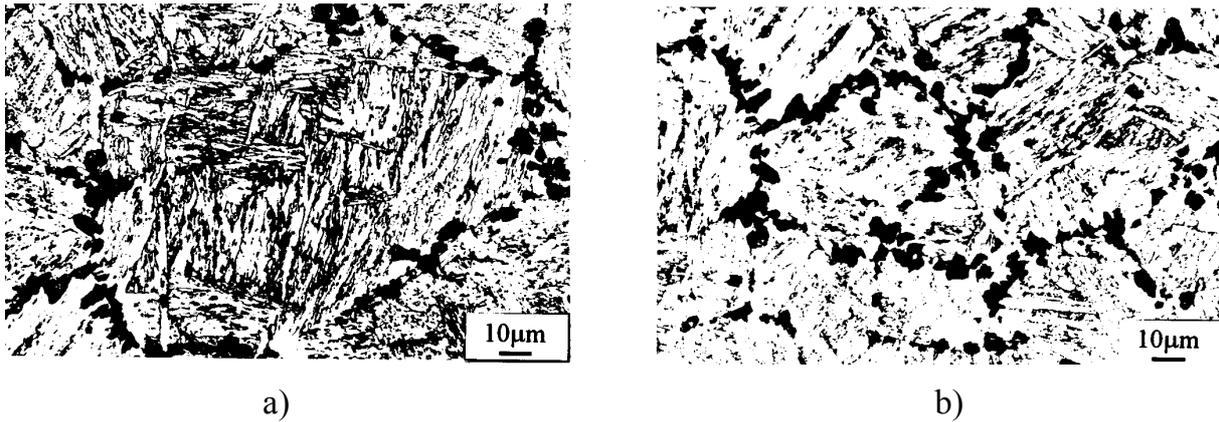
Figure 3. CG HAZ with bainitic - martensitic microstructure, which was subsequently heated at temperature between  $A_{c1}$  and  $A_{c3}$  i.e. IC CG HAZ with distributed brittle M-A constituents along grain boundaries of primary grains (ASTM 4) with directed bainitic microstructure in the HAZ of root region of homogeneous a) and heterogeneous b) under-matched welded joint
