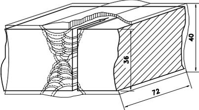
Figure 1. Location of fatigue pre-crack tip in the welded joint
