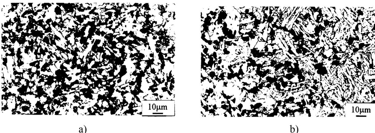
Figure 4. Figure a) shows subsequently heated fine grained microstructure (IC HAZ) at final fracture of specimen with homogeneous weld joint.
