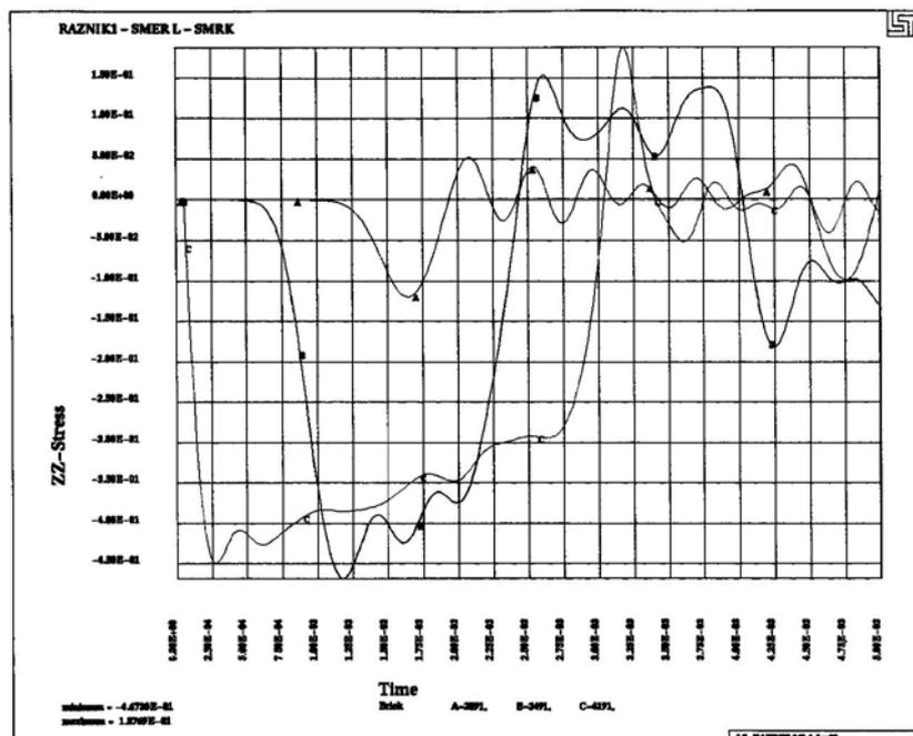
Fig.2. The axial stress component at the specimen axis. Impact velocity  $V = 220$  m/s in the L direction. Projectile thickness has been 2 mm. C denotes the point at 0.25 mm from the loading surface, B denotes the point at 3.75 mm from the loaded surface and A is at 0.25 mm from the free surface.
