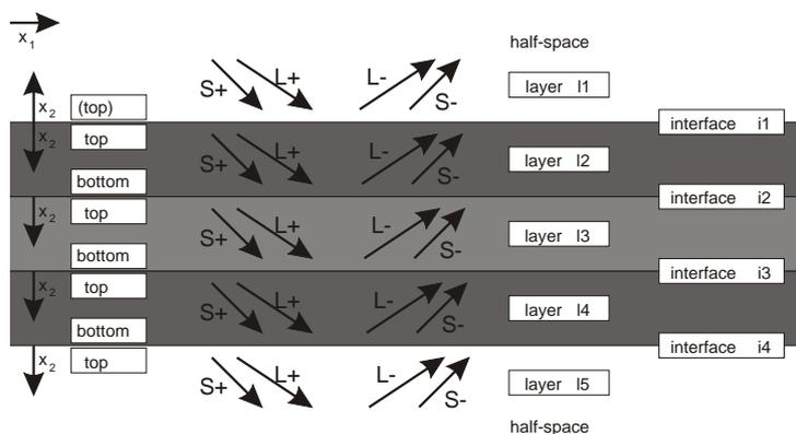
Figure 1: Labeling system for the multilayered plate.
