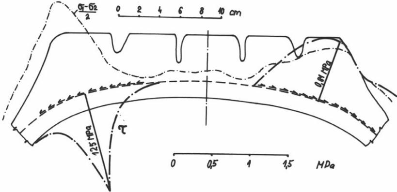
Fig. 6. A radial tyre with lateral force
