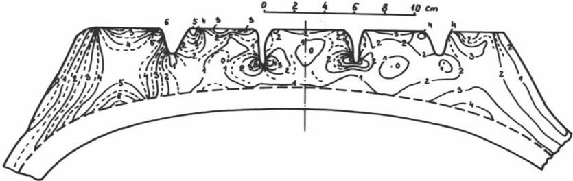
*Fig. 2. A tyre with a radial reinforcement and a lateral force*
