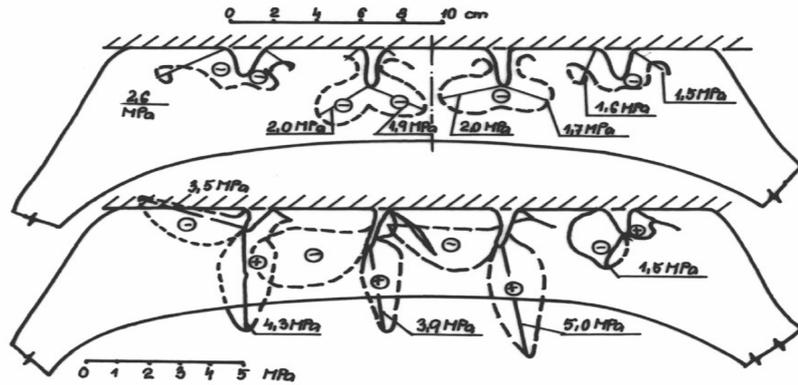
Fig. 3. A tyre with a radial reinforcement and a lateral force in the lower part
