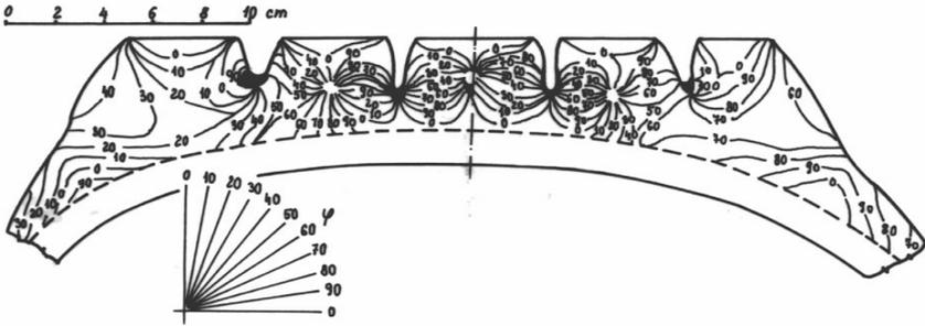
*Fig. 1. A chart of the isoclines in the tyre with a radial reinforcement and asymmetrically deformed by a radial force*
