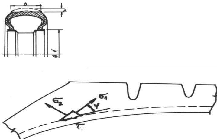
Fig.4. Shear stress along the reinforcing ply
